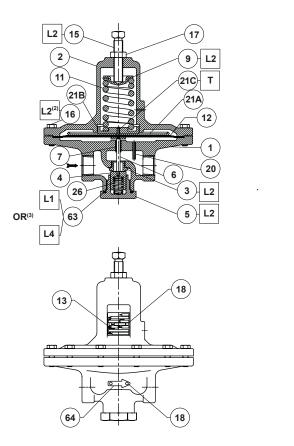
50 SEALED ADJUSTING **SCREW OPTION** 22) L2 **TEE-HANDLE OPTION COMPOSITE SEAT OPTION** 6B 52 6C 6A **CONTROL LINE OPTION** (12 METAL DIAPHRAGM OPTION
